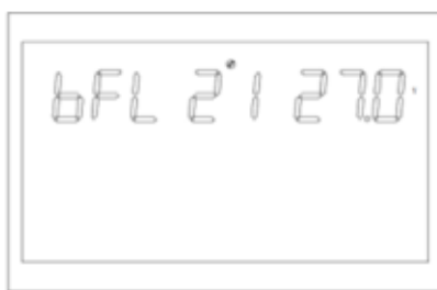
Figure 1-38 Floating charge mode voltage point setting page
