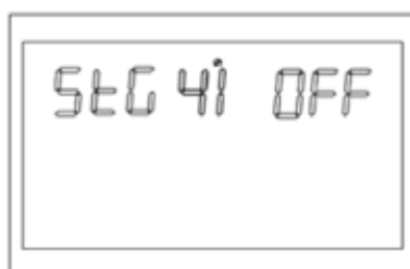
Figure 1-58 Low SOC to mains function setting page
