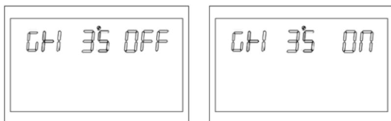
Figure 1-52 The grid-connected inverter function setting page
