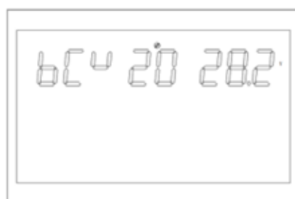
Figure 1-37 Constant voltage mode voltage point setting page
