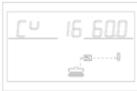
Figure 1-16 Display page sixteen (lithium battery constant voltage information)
