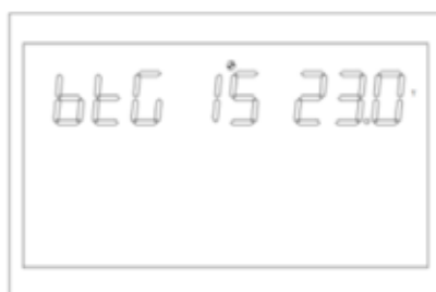
Figure 1-32 Battery mode to mains mode voltage point setting page
