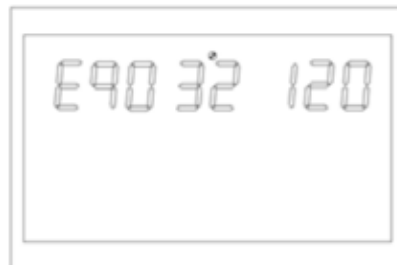
Figure 1-49 Equalization Delay Time Settings Page
