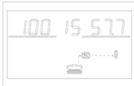
Figure 1-15 Display page 15 (battery capacity information of lithium battery)
