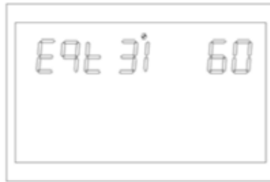
Figure 1-48 Equalization charging time setting(page)
