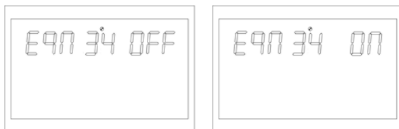
Figure 1-51 Turn on equalization settings immediately
