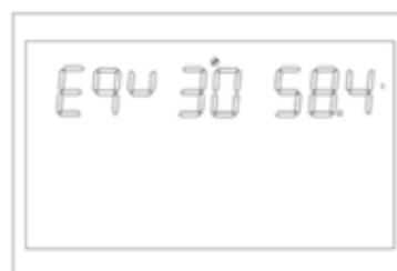
Figure 1-47 Equalization voltage point setting page
