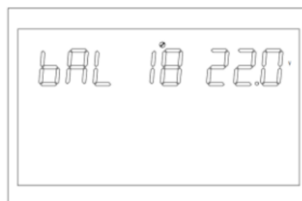
Figure 1-35 Battery low voltage point setting
