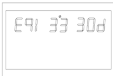
Figure 1-50 Equalization interval setting
