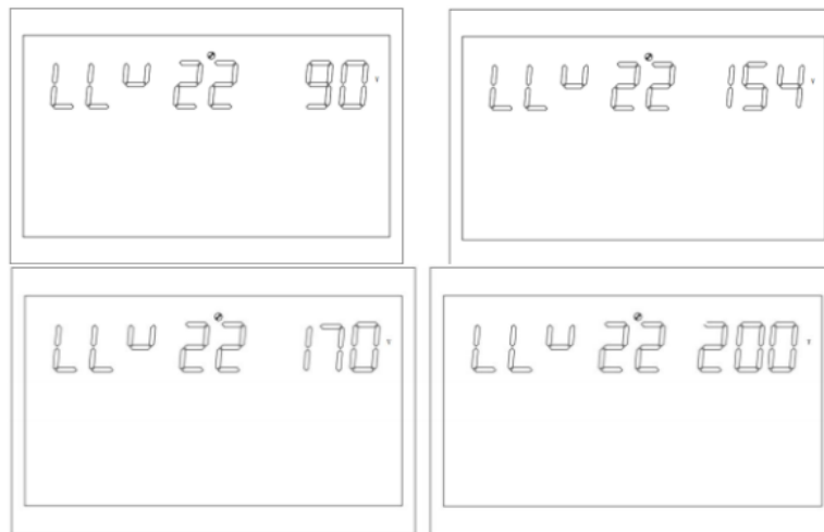
Figure 1-39 Mains low voltage point setting page in APP mode
